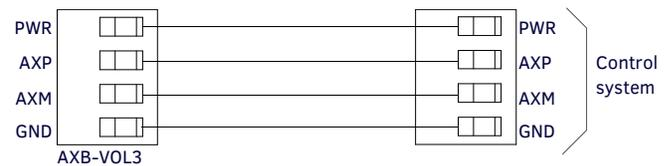
FIG. 3 AXLINK DATA/POWER CONNECTIONS
