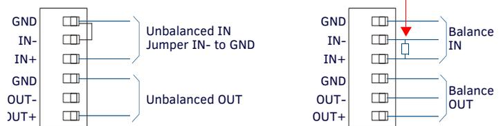
FIG. 4 VOLUME CHANNELS 1 - 3 CONNECTOR WIRING DIAGRAMS
