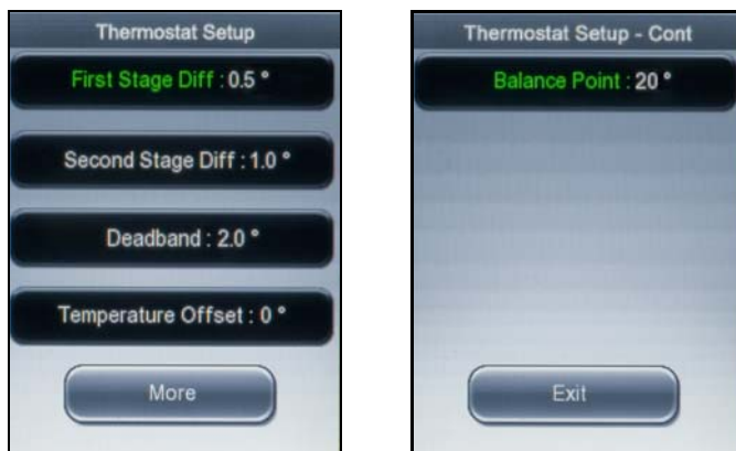
FIG. 47 Thermostat Setup screens
