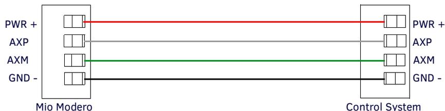
**FIG. 14** AxLink straight-thru wiring
