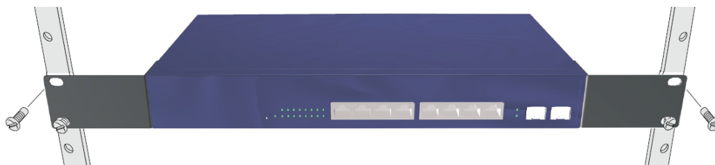
FIG. 17 Installing the Switch in a Rack
