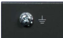
FIG. 7 Rear Panel - Grounding Point
