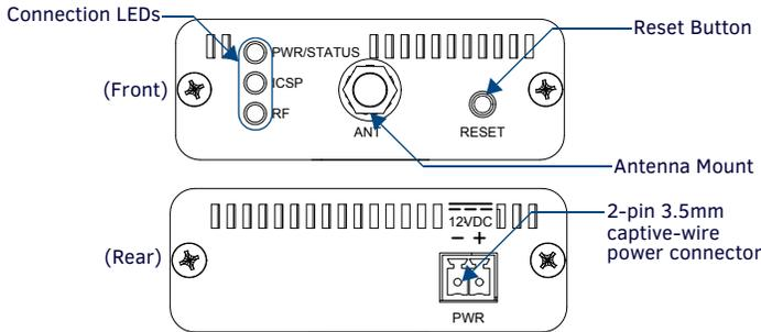
FIG. 1 THE NXR-ZRP-PRO DEVICE (FRONT AND REAR)
