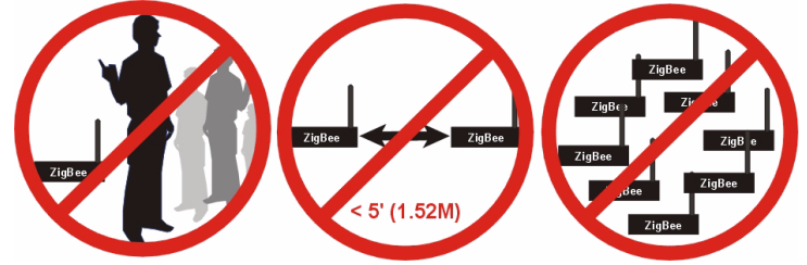
FIG. 3 PROPER PLACEMENT OF ZIGBEE APS
