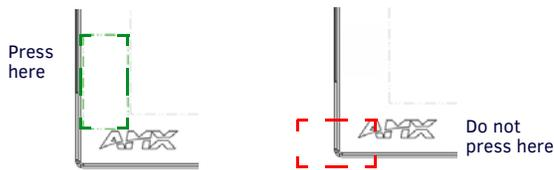
**FIG. 7** PRESS FLAT ON THE CORNER AREA OF THE TOUCH PANEL IN THE APPROXIMATE AREA OF THE CATCHES IN THE WALL FRAME TO LOCK IT IN PLACE (PORTRAIT ORIENTATION DISPLAYED)
