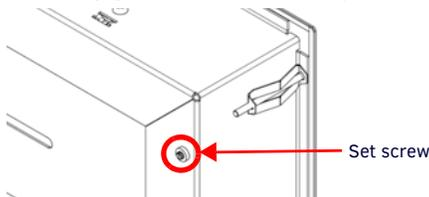
**FIG. 2** SET SCREWS LOCATED ON THE BASE OF THE WALL FRAME, ONE IN EACH CORNER
