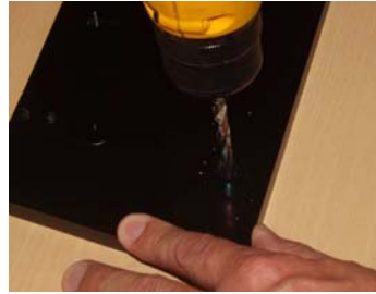
FIG. 2 MARKING THE LOCATION OF THE HEX HEAD BOLT HOLES
