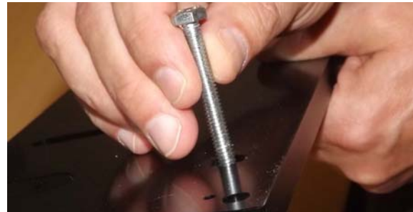
FIG. 4 INSTALLING THE HEX HEAD BOLTS THROUGH THE SECURITY MOUNT BASE
