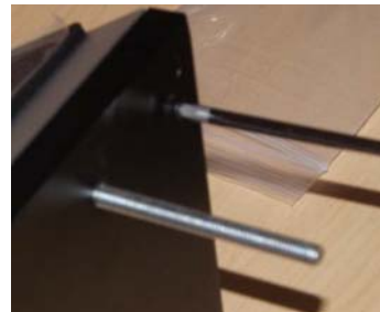
FIG. 5 SECURING THE SECURITY MOUNT BASE TO THE BOTTOM OF THE TOUCH PANEL
