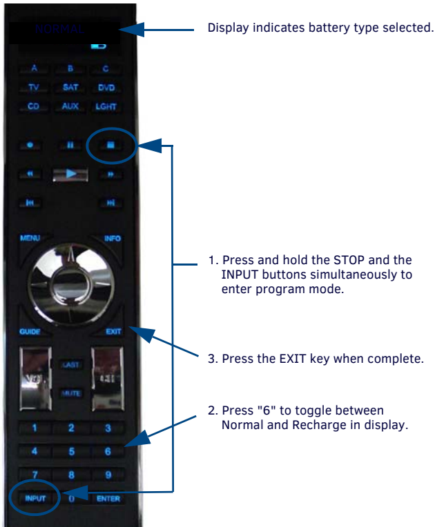
FIG. 4 REMOTE "BATTERY TYPE" PROGRAMMING FEATURES
