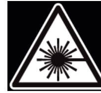
Laser Hazard Symbol label, placed on rear panel, 44 x 38 mm (1.7 x 1.5 in.).
