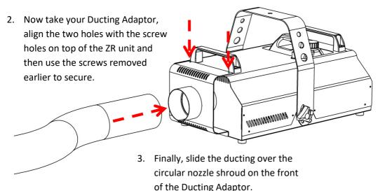
If required: Secure the ducting to the adaptor using a 4" Hose Clip (not included)
