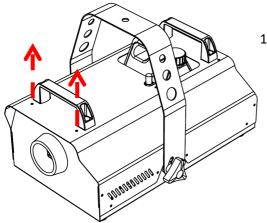
In order to fit the Ducting Adaptor to your JEM ZR25<sup>™</sup>, JEM ZR35<sup>™</sup> or JEM ZR45<sup>™</sup> unit, you will first need to remove the two front screws from the top of your unit.
