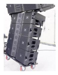
11. Using the integrated rear handle on the VTX-V20-VT, lift the VTX-V20 array until the rear attachment points on the VTX-V20-DF side adapter frames align with the V20-DF main frame.
