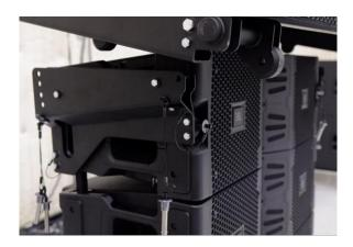
8. Position the suspended VTX-V25-II / V25-II-CS array at a height which aligns the front attachment points on the VTX-V20 side adapter frames at the same height as the front attachment points on the VTX-V20-DF main frame
