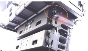
12. Once the rear attachment points have been aligned for the proper angle selection, secure them on both sides with the captive QRP's included on the VTX-V20-DF side adapter panels.
