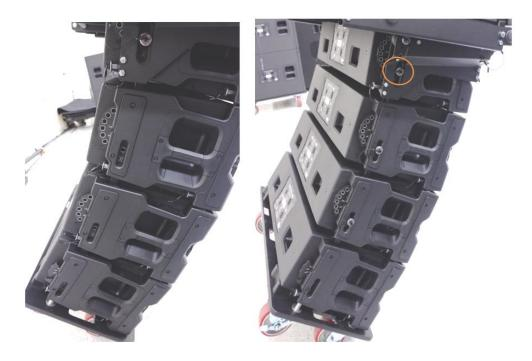
15. Carefully continue lowering the array until the inter-enclosure angles between VTX-V20 cabinets have been completely closed. Use the captive QRP's on each VTX-V20 cabinet to secure the systems in place on both sides of the array at the selected angles. For the top-most VTX-V20, use the captive QRP that is attached to the VTX-V20-DF side adapter frame.
