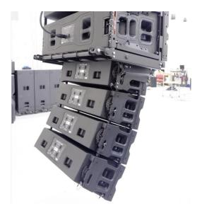
17. At this point VTX-V25-II-CS arrays can be safely compressed. Attach the compression suspension dual-leg chain sling and shackles, then use the VTX V25-LH to compress the array. (Approved OEM factory-approved suspension hardware is available from JBL Professional Customer Service)
