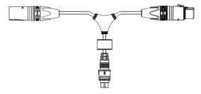
from DMX Source and Tripix Power IP66 towards start of daisy-chain *P/N 11840194 (0.25m)*
