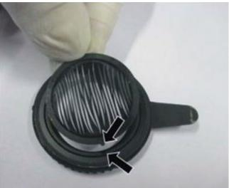
The washer **must be glued** to the custom gobo using a silicone adhesive sealant which bonds to both glass and metals – it must have a high and low temperature resistance from -55 °C to 200 °C (continuous operation)
