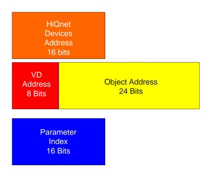
Addressing in HiQnet is split up into three main sections, a 16 bit HiQnet Device address, a 32 bit field that designates the Virtual Device and Object and finally a parameter Address that designates the correct parameter within the Object. The System Explorer in System Architect always shows any of these addresses with a trailing number enclosed in '[]'.
