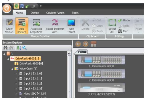
The fully qualified 48 bit address of the first mixer then is [3(Device).0(VD).3.2.0(Object)]
