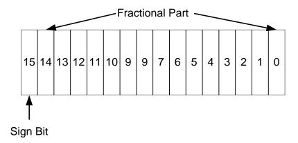
In 1.15 format, bit 15 is used to indicate the sign and the remaining bits 0 to 14 are used to represent the fractional part of the number. 0x8000 represents -1.0 and 0x7fff represents 1.0 - 1/32768. The method uses an implicit scale factor of 100%, so 0x8000 = -100% and 0x7FFF = approximately <math>100%.
