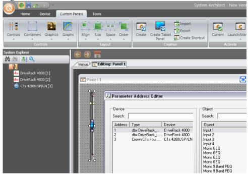
5) The full address is now visible in the Parameter Address Window. In this example, this is HiQnet Address 3, Virtual Device 0, Object Address [5.40.1] and Parameter Index 0.
