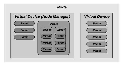
The HiOnet product is modeled with a multi-tiered approach. The top level that usually represents the product itself is called a Device. The Device must contain at least one Virtual Device, the first of which acts as a Device Manager. Each Virtual Device can contain Objects and/or Parameters. Objects themselves can contain other Objects or Parameters. A Parameter contains the state of a single controllable variable. Below we will define each of these terms in detail.
