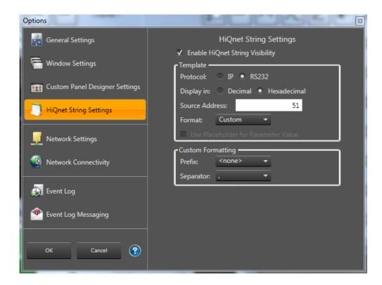
Make sure that "Enable HiQnet String Visibility" is checked. This turns on the feature.
