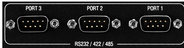
FIG. 18 RS-232/422/485 Device Port connectors
