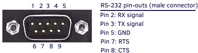
FIG. 6 RS-232 (DB9 - Male) Connector Pin-outs
