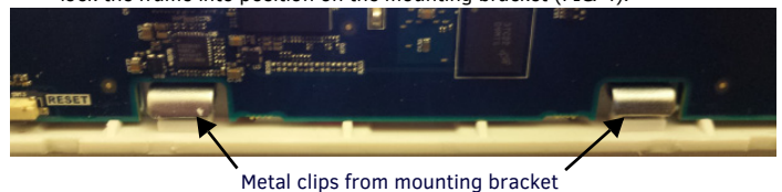
FIG. 4 METAL CLIPS FROM MOUNTING BRACKET LOCKING FRAME ONTO BRACKET
