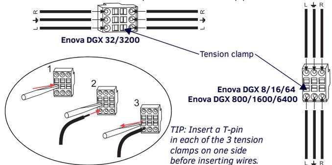
**FIG. 8** AUDIO WIRING FOR AIE BOARD
