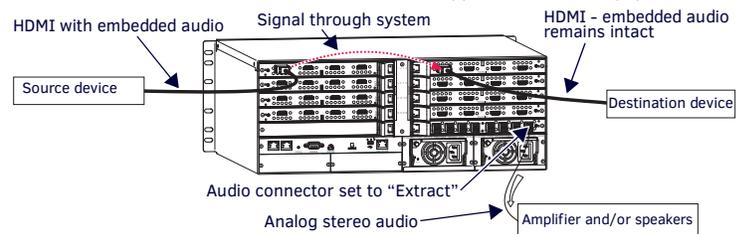
**FIG. 4** AUDIO EXTRACTED FROM HDMI OUTPUT SIGNAL
