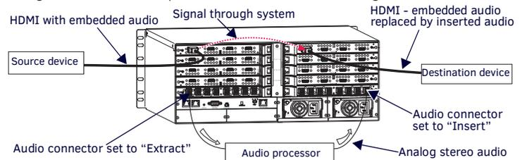
**FIG. 5** AUDIO EXTRACTED FROM HDMI INPUT SIGNAL AND INSERTED ONTO HDMI OUTPUT SIGNAL
