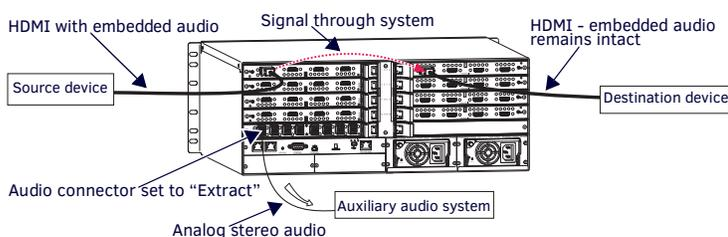
**FIG. 1** AUDIO EXTRACTED FROM HDMI INPUT SIGNAL AND SENT TO AUXILIARY SYSTEM
