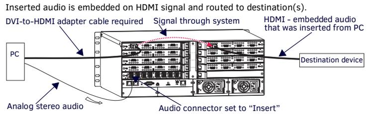
**FIG. 2** AUDIO INSERTED ONTO HDMI INPUT SIGNAL
