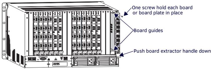
**FIG. 6** REMOVE SCREW, PUSH BOARD EXTRACTOR HANDLE DOWN, THEN PULL BOARD STRAIGHT OUT (ENOVA DGX 32 SHOWN)
