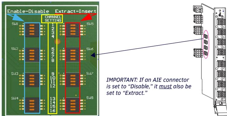
**FIG. 7** AIE BOARD AND DIP SWITCHES
