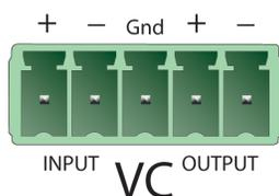
FIG. 7 VC Connector Pin-out
