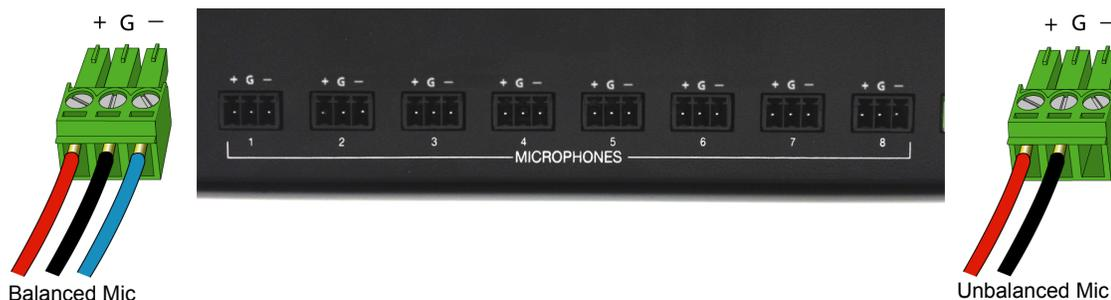
**FIG. 21** Microphone Connection Wiring
