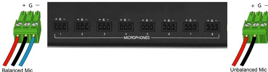
**FIG. 21** Microphone Connection Wiring
