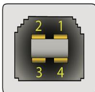
**FIG. 12** USB Port Pin-out
