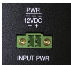
FIG. 17 12-Volt Power Connection
