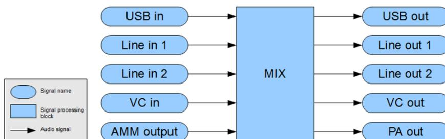
**FIG. 2** Mixing of Processed Microphone Channels with Input to Form Output Signals
