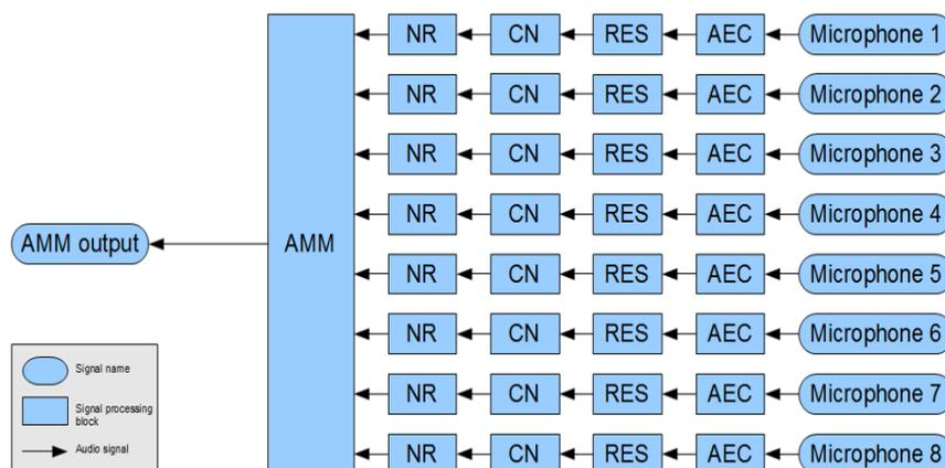
**FIG. 1** Microphone Signal Processing Flowwebpage
