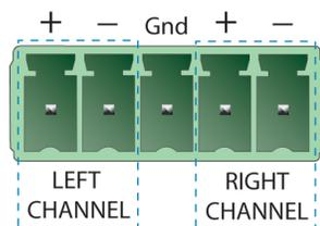
**FIG. 9** PA Speaker Connector Pin-out
