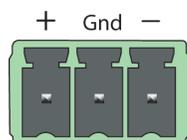
**FIG. 10** Microphone Input Pin-out
