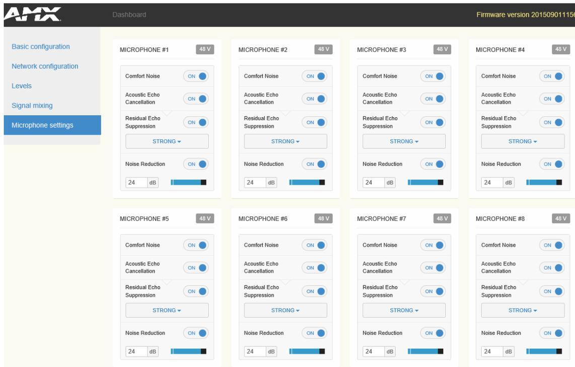
**FIG. 30** Configuration of Signal Processing Applied to Microphone Signals.
