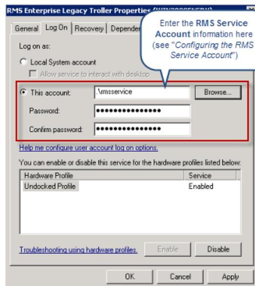
FIG. 43 RMS Enterprise Legacy Troller Properties dialog (Log On tab)
