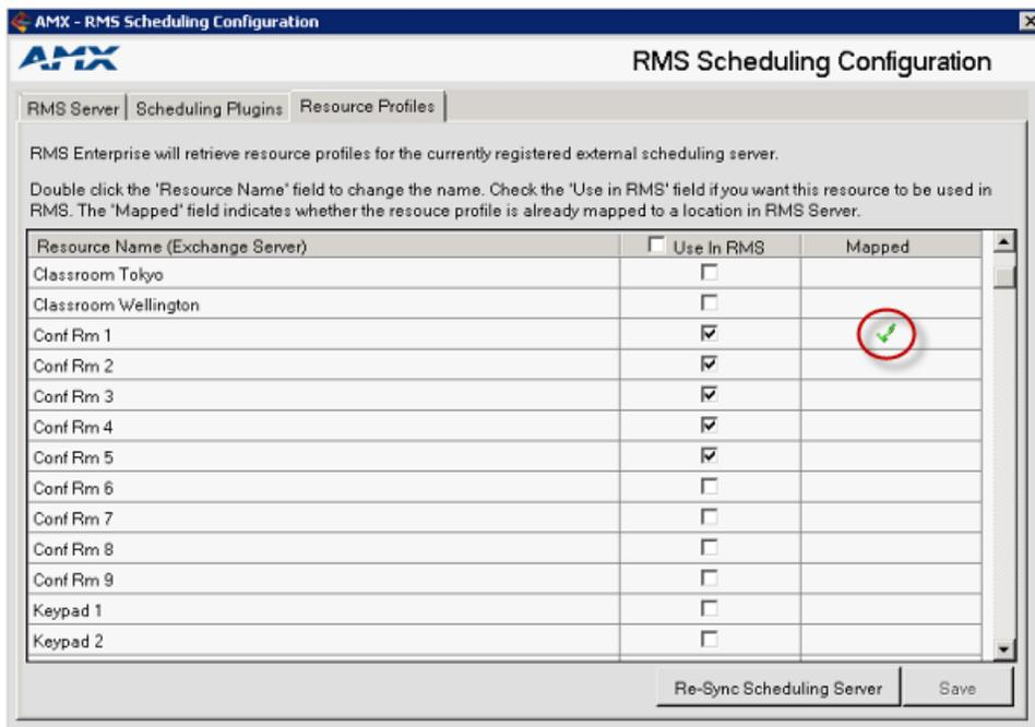
FIG. 48 RMS Scheduling Configuration application (indicating "ConfRm1" mapped)
