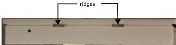
**FIG. 5** LOCATION OF RIDGES ON BOTTOM OF MKP-106
