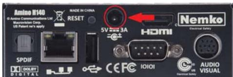
FIG. 100 STB-04 - Rear Panel Power Connector
