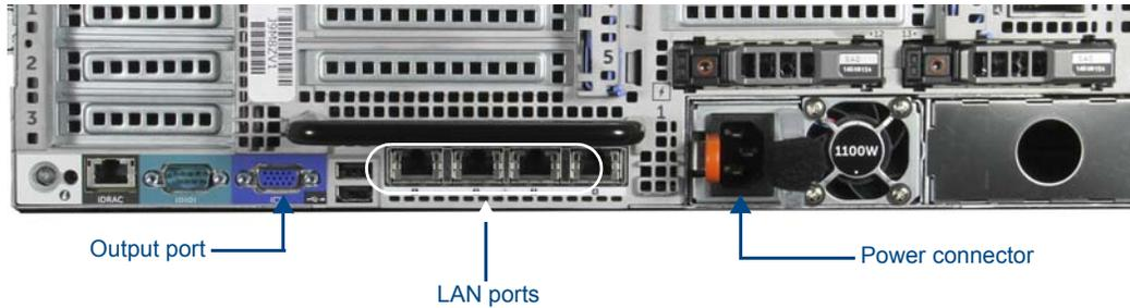
**FIG. 2** Vision<sup>2</sup> Master Server Rear Panel
