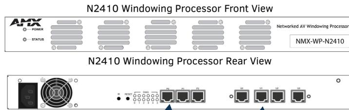
To avoid creating a network loop, connect *only one* of the P ports to the same network switch.
