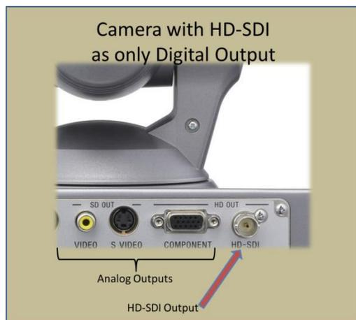
switching and transport layer without the need for additional signal or format conversion. In many cases, devices such as VTC cameras will offer both variants of video outputs. (See image)
