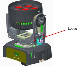
Loosen the 4 screws (marked in red)
