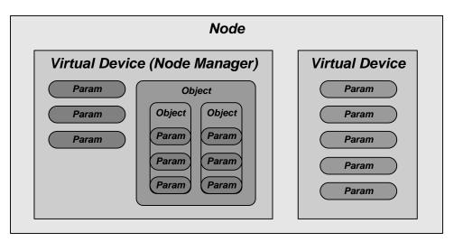
The HiQnet product is modeled with a multi-tiered approach. The top level that usually represents the product itself is called a Device. The Device must contain at least one Virtual Device, the first of which acts as a Device Manager. Each Virtual Device can contain Objects and/or Parameters. Objects themselves can contain other Objects or Parameters. A Parameter contains the state of a single controllable variable. Below we will define each of these terms in detail.
