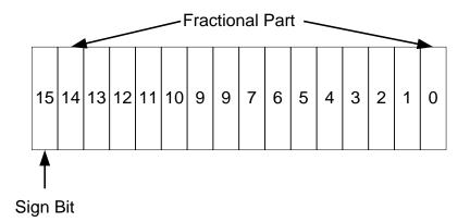
In 1.15 format, bit 15 is used to indicate the sign and the remaining bits 0 to 14 are used to represent the fractional part of the number. 0x8000 represents -1.0 and 0x7fff represents 1.0 - 1/32768. The method uses an implicit scale factor of 100%, so 0x8000 = -100% and 0x7FFF = approximately 100%.
