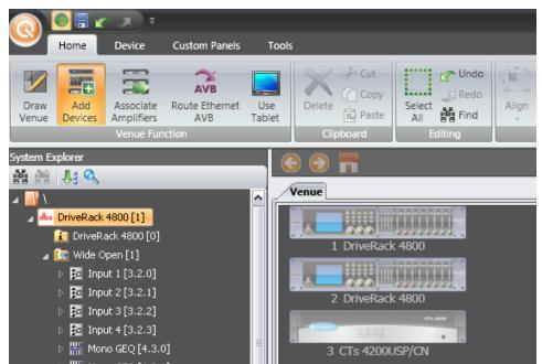
The fully qualified 48 bit address of the first mixer then is [3(Device).0(VD).3.2.0(Object)]
