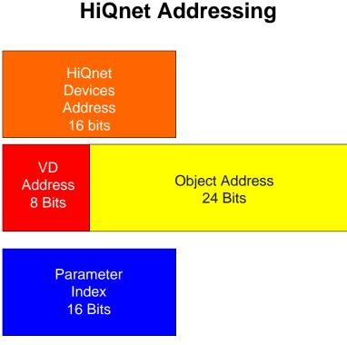
Addressing in HiQnet is split up into three main sections, a 16 bit HiQnet Device address, a 32 bit field that designates the Virtual Device and Object and finally a parameter Address that designates the correct parameter within the Object. The System Explorer in System Architect always shows any of these addresses with a trailing number enclosed in '[]'.
