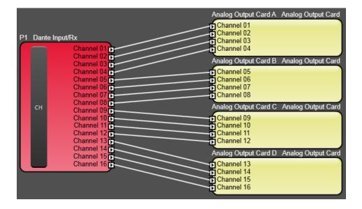
Shown above is one of the BLU-326 devices configured as one of the twelve output modules. The Dante processing object is configured as an input from the Dante network and then distributes the 16 signals to the analog outputs.
