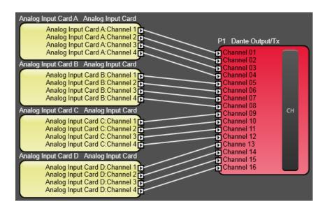
Shown above is the signal routing from one BLU-326 configured as one of the four input modules to an Dante processing object. The processing object has been configured to accept the 16 channels of audio and put them onto the Dante network.
