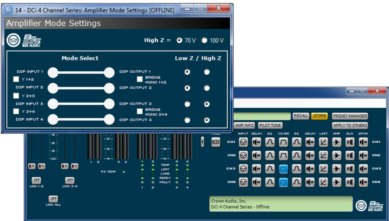
**Step 6:** Once you have the correct High Z modes selected you are ready to send the settings to the amplifier. Click on the Go Online button in the Offline Design → Workflow ribbon as shown below.
