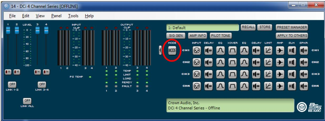
**Step 4:** In the upper right corner of the Amplifier Mode Settings window you will see the global High Z voltage setting. Select the voltage setting that is required for the High Z speakers in the audio system, either 70V or 100V. This setting is global for all channels set to High Z.
