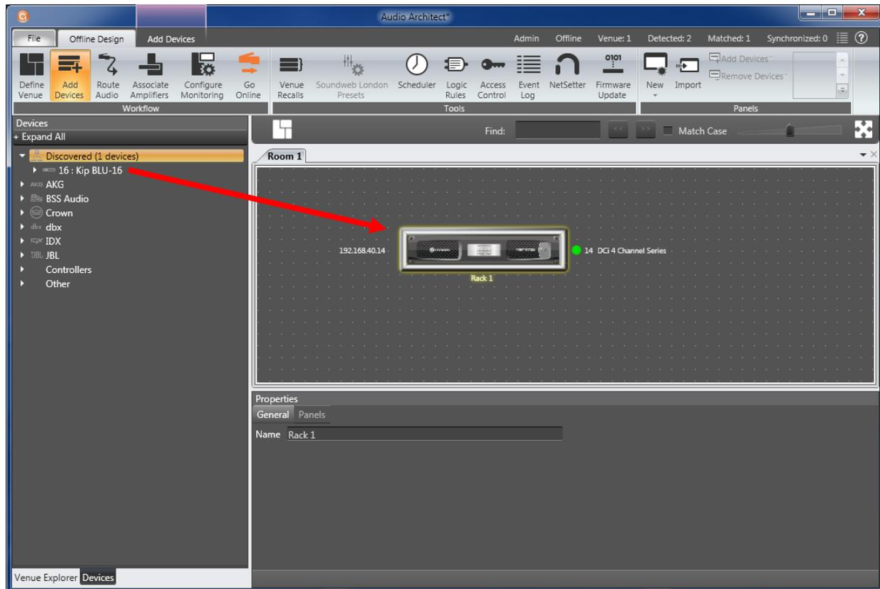
**Step 2:** Double click on the amplifier to open the Default Device Panel.
