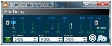
The Delay Block contains a signal delay display. You may enter the delay in either milliseconds, feet, or meters.
