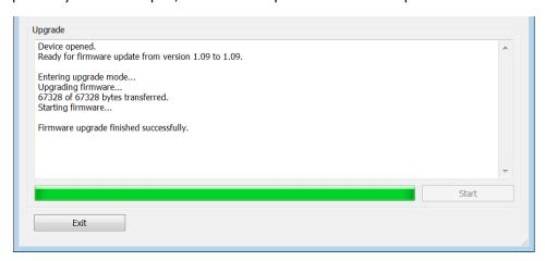
After successful firmware update, the Notepad should be power-cycled to ensure it is detected by the computer's USB interface before using for audio. Note that the 'Current Firmware' may not display the new version number until the console is power-cycled.
