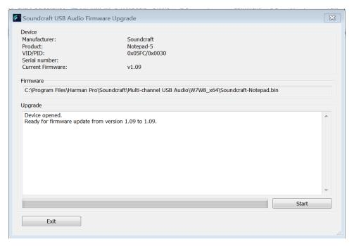
Click the Start button in bottom right of Firmware Upgrade window. A progress bar will be displayed and show a notification when successfully complete (see screenshot below).
