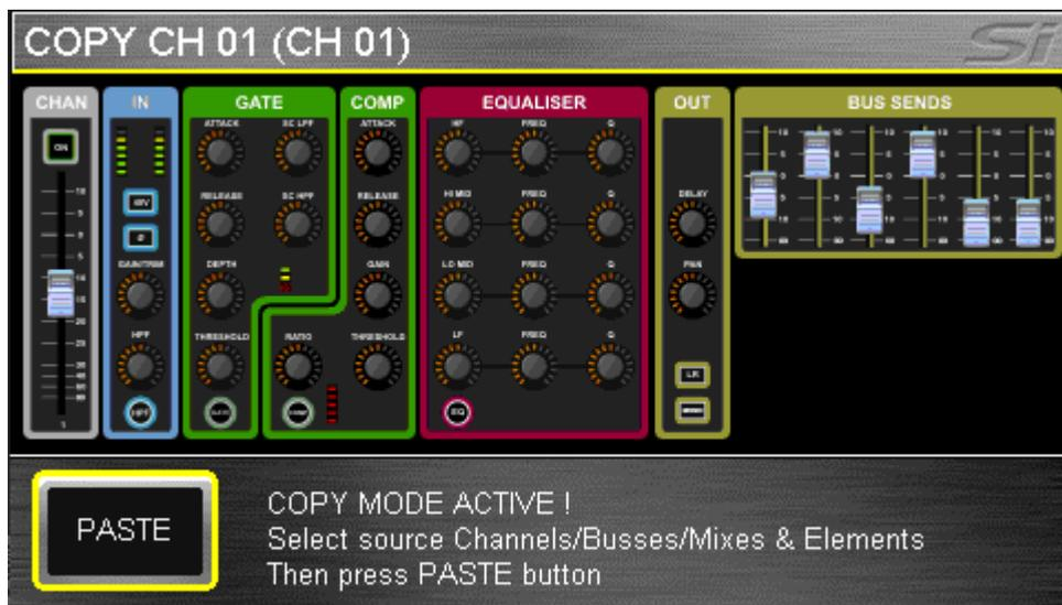
Pressing and holding the PASTE Hold button (or the latching PASTE on the Offline Editor) will open the PASTE MODE screen and the user is requested to select the target channels/busses.
