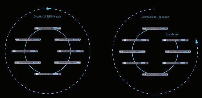
BLU link audio can be transmitted from device to device with a maximum CAT-5e cable length of 100 metres (328 ft). It can also be converted to fiber for much longer runs with the BSS Audio MC-1 media converter. A maximum of 60 BLU link devices may be connected in a single ring.
