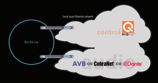
Perhaps one of the most practical uses of the combination of an Ethernet transport network and BLU link is using a central Ethernet network cloud to transmit audio between racks or even between rack rooms, and then distribute audio locally with several BLU link rings within the rack or room:
