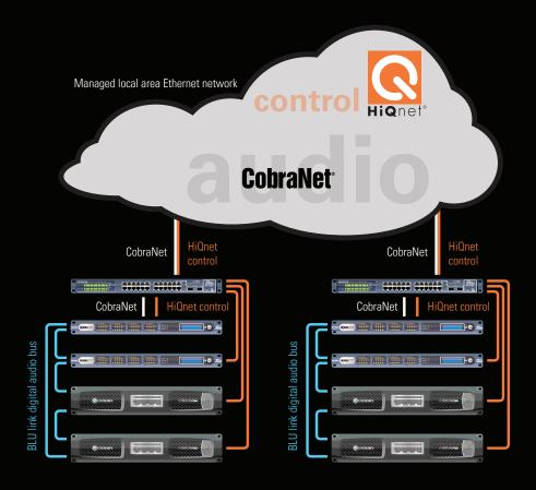
In the diagram, audio is distributed across the facility from and to BSS Audio Soundweb London devices in rack rooms. Within each rack room audio is distributed to other Soundweb London devices and Crown amplifiers using BLU link. The BLU link bus has the capacity to distribute all of the channels within the rack room — including redistributing CobraNet audio, as well as any additional audio that only needs to be sourced and distributed locally between the devices in the rack.
