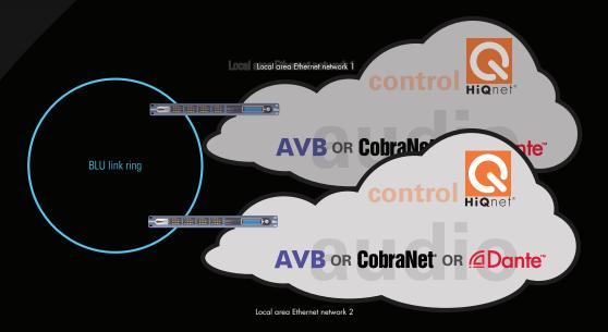
The system above must therefore be fixed by connecting the two Ethernet transport networks together so they share the same clock, even though there may be no audio passing between them:
